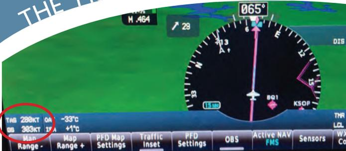
**AVL to ESN:** 370 NM, 1.4 hours, FL 250, -32C, 1550 TO, 785 Degrees C ITT, 330 lbs per hour fuel flow, **282 KTAS**
