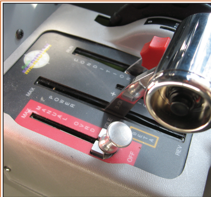
The engine control quadrant of a Piper Meridian
