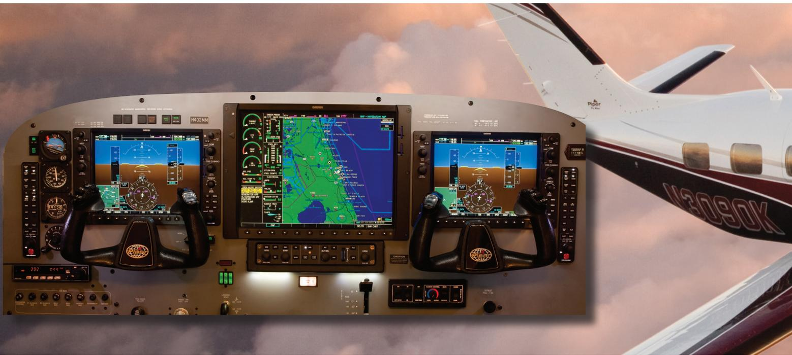
2006 models, comprised of pilot and copilot Primary Flight Displays (PFDs), a center Multi-Function Display (MFD) and dual Garmin 430’s for GPS/COMM/NAV. The simplicity of operation coupled with large displays, and the features they provided, afforded owners with capabilities not only similar to larger business jets, but in some cases better. The Avidyne set-up left many asking the question: “What could possibly be next?” or “How can this get any better?” Enter the Garmin G1000 Meridian.
