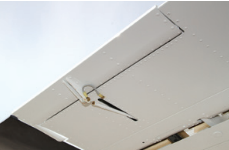
>>> One of the upgrades in the NG model is the addition of servo tabs on the ailerons, which provide better roll response.
