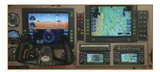
• An Avidyne Entegra flat panel, two screen display system. The EXP5000 Primary Flight Display (PFD) will portray all operational, navigation and flight parameters. The multi-function display will portray moving map, trip information, engine display parameters and system monitoring. The Avidyne MultiLink system features Sirius Satellite radio, satellite weather datalink with weather graphics displayed on the MFD.
