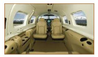
• A roomy cabin, with airstair entry door on the port side of the fuselage, has the current Piper Meridian interior scheme. Four leather-upholstered seats are placed in a club arrangement with a retractable executive writing table. There is an open storage area between the cockpit and the rear-facing seats. An off-white headliner and window panels, with color-coordinated carpeting and side panels are installed, with your choice of two interior color schemes.
