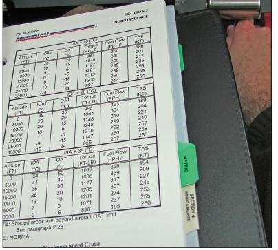
Operating the engine beyond the recommended power settings in the POH / AFM for a prolonged period will result in accelerated margin deterioration due to hot section component distress and will affect engine reliability and durability. This effect is cumulative and will lead to the engine prematurely reaching an operating limit (usually ITT) before the recommended power is produced."
