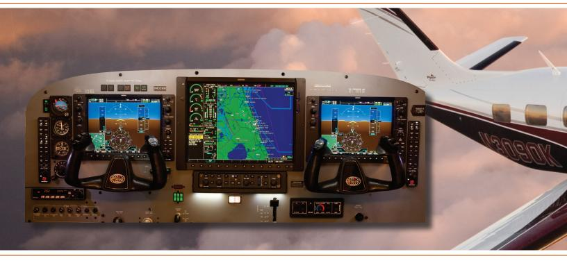
2006 models, comprised of pilot and copilot Primary Flight Displays (PFDs), a center Multi-Function Display (MFD) and dual Garmin 430's for GPS/COMM/NAV. The simplicity of operation coupled with large displays, and the features they provided, afforded owners with capabilities not only similar to larger business jets, but in some cases better. The Avidyne set-up left many asking the question: "What could possibly be next?" or "How can this get any better?" Enter the Garmin G1000 Meridian.
